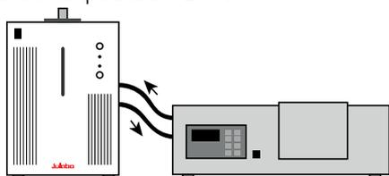
AWC100 is designed to cool water in closed loops. The unit permanently removes heat from water as it flows through the machine.
