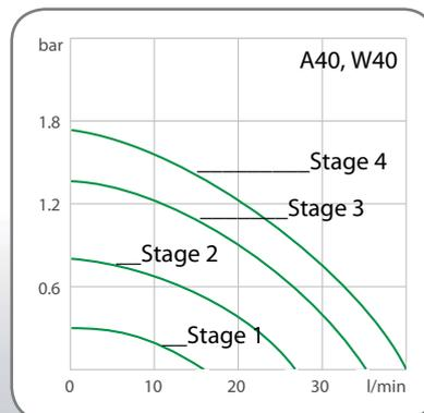
All data refers to the nominal voltage of 230 V, nominal frequency of 50 Hz and ambient temperature of +20 °C. Cooling capacity measured at max. pump stage. All pump data refers to a bath fluid with a specific density of 1 kg/dm<sup>3</sup>. Cooling capacity measured with Thermal HL (+200 °C) or Ethanol (except +200 °C)
