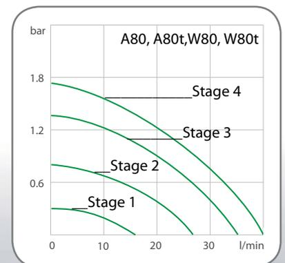
All data refers to the nominal voltage of 230 V, nominal frequency of 50 Hz (respectively 400 V, 3Ph., 50 Hz) and ambient temperature of +20 °C.
