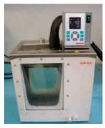
only forming at the outher parts of the glass window. Only when going below -40 °C the sight was inhibited by a stronger formation of ice. As a summary one can say that the combination of an ME-18V with an immersion cooler Ft900 is an efficient and economic way for viscosity measurement at low temperatures.
